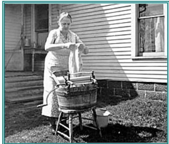
Figure 42 Manual washing machine with wringer
